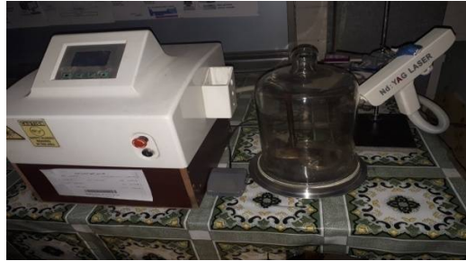
Figure(1) shows system of PLD
